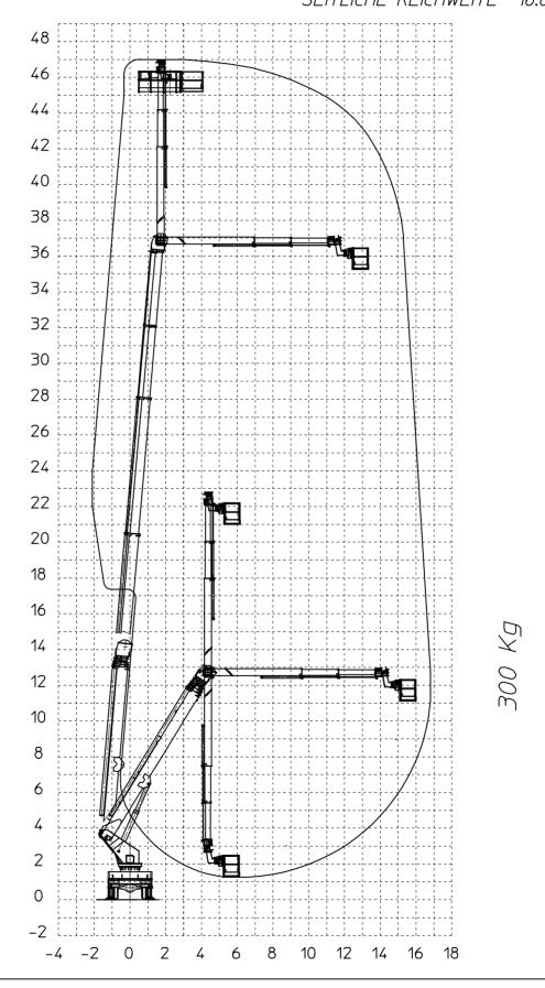
MULTITEL J346TA/S Ente Rev. Data Dis. Contr. Ap.AQ Descrizione EMISSIONE 16-04-03 W.B. DIAGRAMMA - SCHEDA 54/2 - Rev. 0 - 15/12/00 D34135 SBRACCIO DI LAVORO 27.5 m ±5% WORKING OUTREACH 27.5 m ±5% DEPORT DE TRAVAIL 27.5 m ±5% SEITLICHE REICHWEITE 27.5 m ±5% 44 42 40 38 36 34 32 30 28 26 24 22 20 18 16 14 12 10 8 4 2 0 -2 -4 -6 -8 -10 -12
